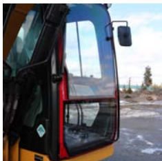
UL752 Level 1 Ballistic Window.
