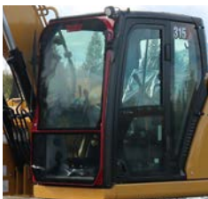
Our polycarbonate excavator windows have not been drilled or milled making it less susceptible to micro-fractures and is bonded to a steel frame making it flex less.
