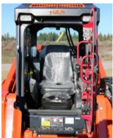
Our polycarbonate skid steer doors have not been drilled or milled making it less susceptible to micro-fractures and is bonded to a steel frame making it flex less.
