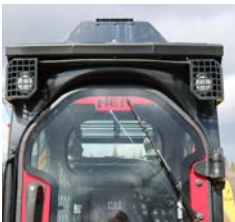
Our polycarbonate skid steer doors have not been drilled or milled making it less susceptible to micro-fractures and is bonded to a steel frame making it flex less.
